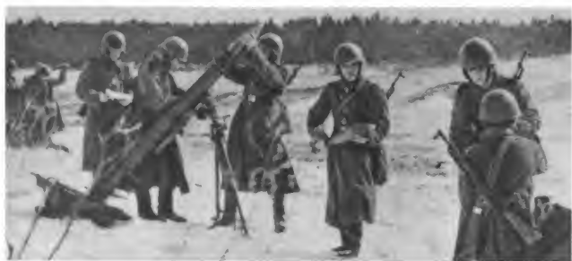
Figure 6-31. Mortars. The standard mortar in Soviet service is the 120-mm medium mortar (above), with a range of 5,700 meters. It is generally replacing the lighter 82-mm mortar (below) in motorized rifle regiments and battalions.
